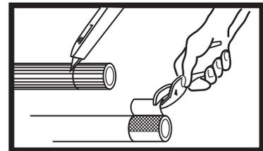
3. After slitting the rubber cover, twist off with pliers. If any particles of rubber remain, remove with wire brush.
