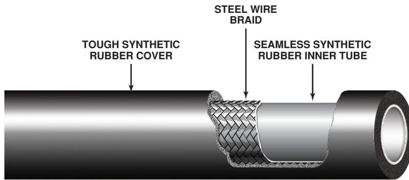
**Z CONSTRUCTION:** Fuel and oil-resistant seamless synthetic rubber tube, single steel wire braid – Skive Type
