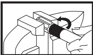
4. Place socket in vise and screw hose in counter clockwise, using body weight against hose to start threading. Tighten until hose bottoms.
