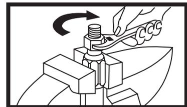
6. Screw nipple into socket, using wrench on hex of nipple. After assembled, blow air pressure to remove any hose particles and inspect.
