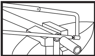
1. Cut hose square to desired length using fine tooth hack saw or cut-off saw.
