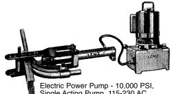
Electric Power Pump - 10,000 PS Single Acting Pump, 115-230 AC Dual Voltage, 3/4 H.P. Single Phase, 64 lbs. Attachments for the Lenz 1880 Hydraulic Tube Bender are shown as Part Numbers in the table above and consist of Radius Shoe, Follow Bar and Saddle.
