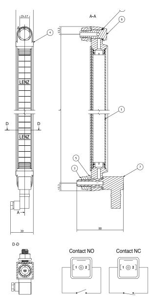
The electrical sensor is stamped N/A (normally closed) or N/O (normally open) and also marked  $60^{\circ}C$  (148°F) or  $70^{\circ}C$  (158°F) for switching temperature.
